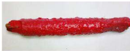
Non-Crosslinked Cable after 1 hour @200 °C
