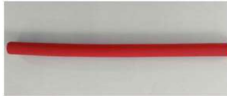
Non-Crosslinked Cable after 1 hour @200 °C
